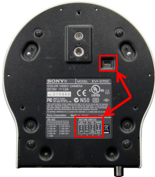
Figure 1: Set the DIP switches on the bottom of the camera.
