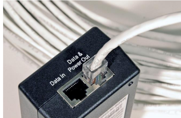
Figure 8: Attach the 100 ft. White CAT5 cable to the AC to DC Power Converter.
