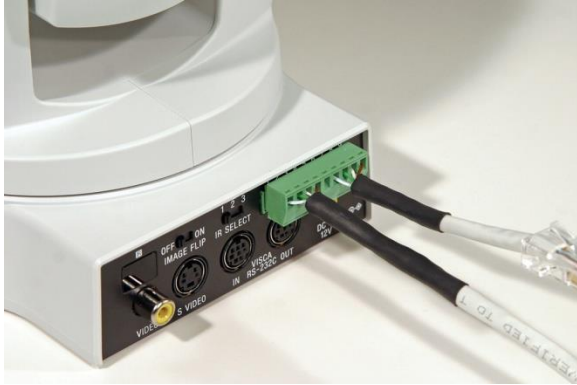
Figure 3: Attach the Green Phoenix Connector Cable to the back of the camera.
