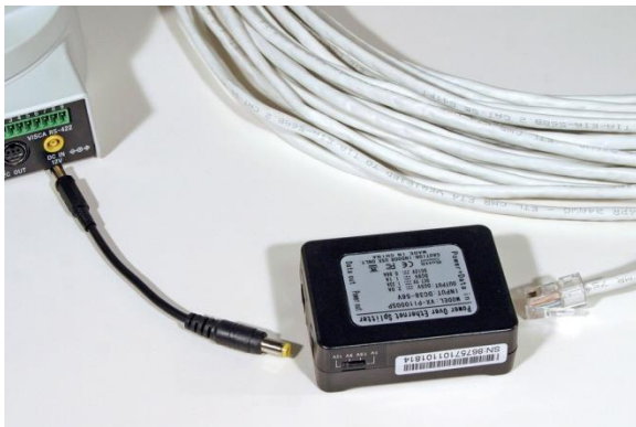
Figure 7: Connect the Power Adapter Cable to the DC Power Input on the back of the camera. Connect the DC Power Supply to the Power Adapter Cable. Connect the DC Power Supply to the CAT5 cable.
